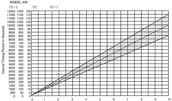
Value Of External Timing Resistor In Meg Ohms
