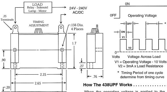
When the operating voltage is applied to the series combination of the 438UPF and the load circuit, the 438UPF turns ON, and the load will be energized. It is important to understand that the load current that flows is determined by the (Applied Voltage - 10 volts) divided by the load resistance. The 10 volts is the maximum voltage that will be dropped across the 438UPF at any operating voltage. As an example: a  $440\Omega$  (ohm) relay coil that would normally draw 250mA at
