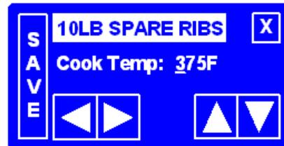
The Cook To Temp is only available if enabled by DIP switches 4 & 5. A standard temperature editing screen is shown above illustrating the ease of adjustment. The recipe name being edited is highlighted, the left and right arrows are used to select the underlined digit to be changed, the up and down arrows change the digit as desired. Pressing the SAVE area saves the changed parameter, pressing X aborts any changes
