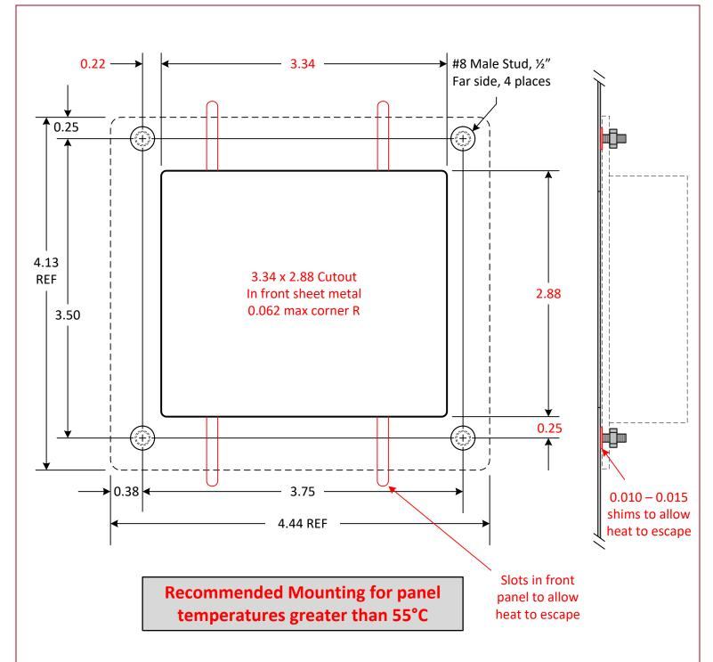
Shims on the mounting studs or slots in the front metal should be used to allow hot air that is trapped between the controller and the overlay to escape. A larger opening for the display is required to increase the distance between the hot front panel and the touchscreen and to allow for additional overlay flexing if shims are used to create the convective cooling required.
