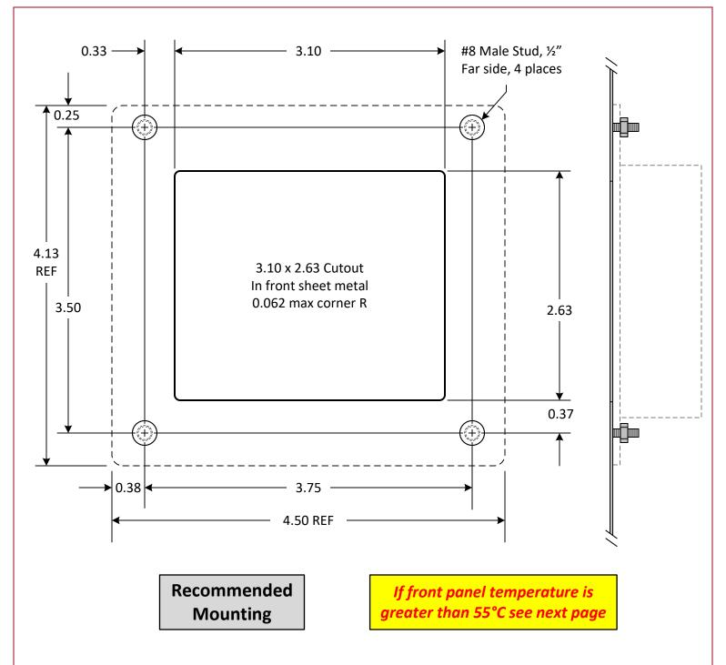
When designing the mounting method with a protective overlay there should be a 0.010'' - 0.015'' gap between the back of the overlay and the front surface of the display. Dielectric dots on the back of the overlay are recommended to prevent adhering of the back of the overlay to the LCD display
