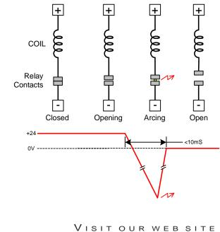
As the contacts start to open the normal current flow through the load shuts off, and the stored inductive energy must now discharge. As the open relay contacts are a high resistance to current flow, the voltage across the load increases quickly in the negative direction (remember the reverse polarity of the stored energy) until the voltage is high enough to jump the air gap between the contacts. This is just like the arc created in spark plugs and happens in a few thousandths of a second.
