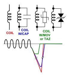
Suppression of inductive load spikes on AC coils is more difficult due to the constantly changing polarity of the load current. There are two basic type of components which can be used:
