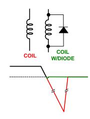
Suppression of inductive load spikes on DC coils is simpler than on AC coils for the simple reason that the current flow through the coil is in only one direction. Connection of a diode with the cathode (striped end) towards the positive side of the coil easily supresses the voltage spike.
