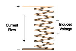
Any coil of wire with current passing through it stores energy in reverse polarity to the flow, this is an inesapable law of basic physics. This is true for both DC and AC coils, the only difference is that the AC current changes polarity 60 times per seconds therefore this stored energy is also changing polarity.
